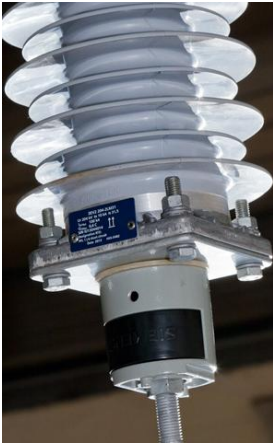
Figure 11 : Fault indicator before short circuit test
