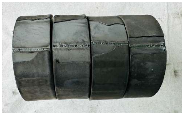
Figure 4. MOV Block Failure Probably Due to Internal Stress from Non-Uniform Sintering. Source TenneT Netherlands.
