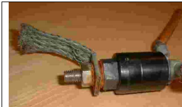
Figure 20. Broken ground lead disconnecter NGLA (5)
